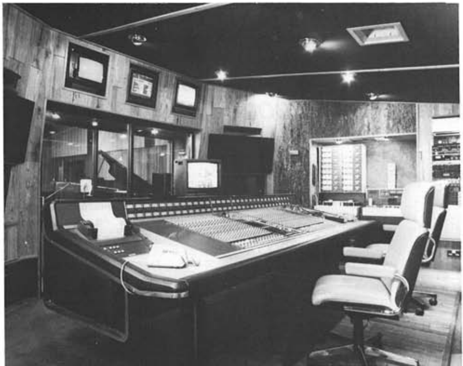
The present recording studio - the Eastlake-designed control room houses a solid state logic computer controlled mixing console. All functions of the console are monitored by the computer which allows total recall of the control settings.
